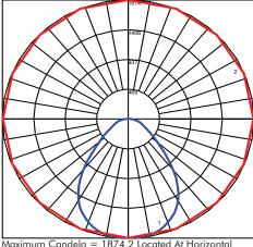
Maximum Candela = 1874.2 Located At Horizontal Angle = 67.5, Vertical Angle = 2.5 # 1 - Vertical Plane Through Horizontal Angles (67.5 -247.5) (Through Max. Cd.) # 2 - Horizontal Cone Through Vertical Angle (2.5) (Through Max. Cd.)
